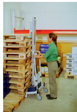
A special version of TAWI Protema PRO70 electric lifter has also been developed for Systembolaget. A forked tool lifts empty pallets after depalletisation.
