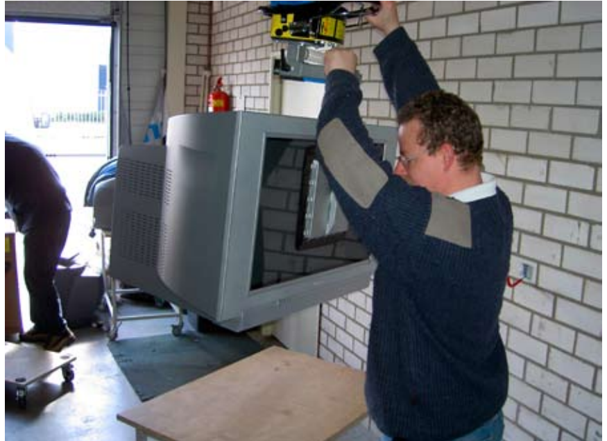
Project nr 2598. A side lifter for TV sets with adjustable suctionfoot. The suction foot is "low-built" to allow passage way into boxes to pick up the sets. On VM160 with fixed handle.
