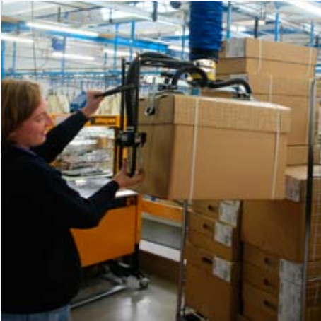
1. Flexible, extended handle turns "over-the-shoulder"-lifting into ergonomic lifting.
