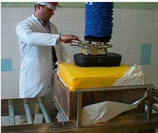
4. A VM160 cheese lifting application for blocks of cheese weighing appr 60-70 kg. Food industry have been using vacuum lifters to handle food stuffs in the cold packaging area for many years.
