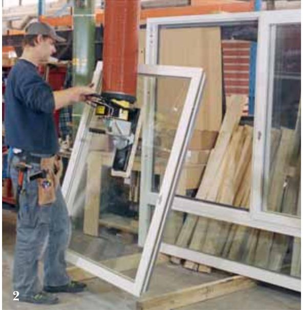
3. Low headroom and more or less no operating space? The VacuEasylift transformed the task of moving 60 kg panels to a punching machine into a one-man job.
